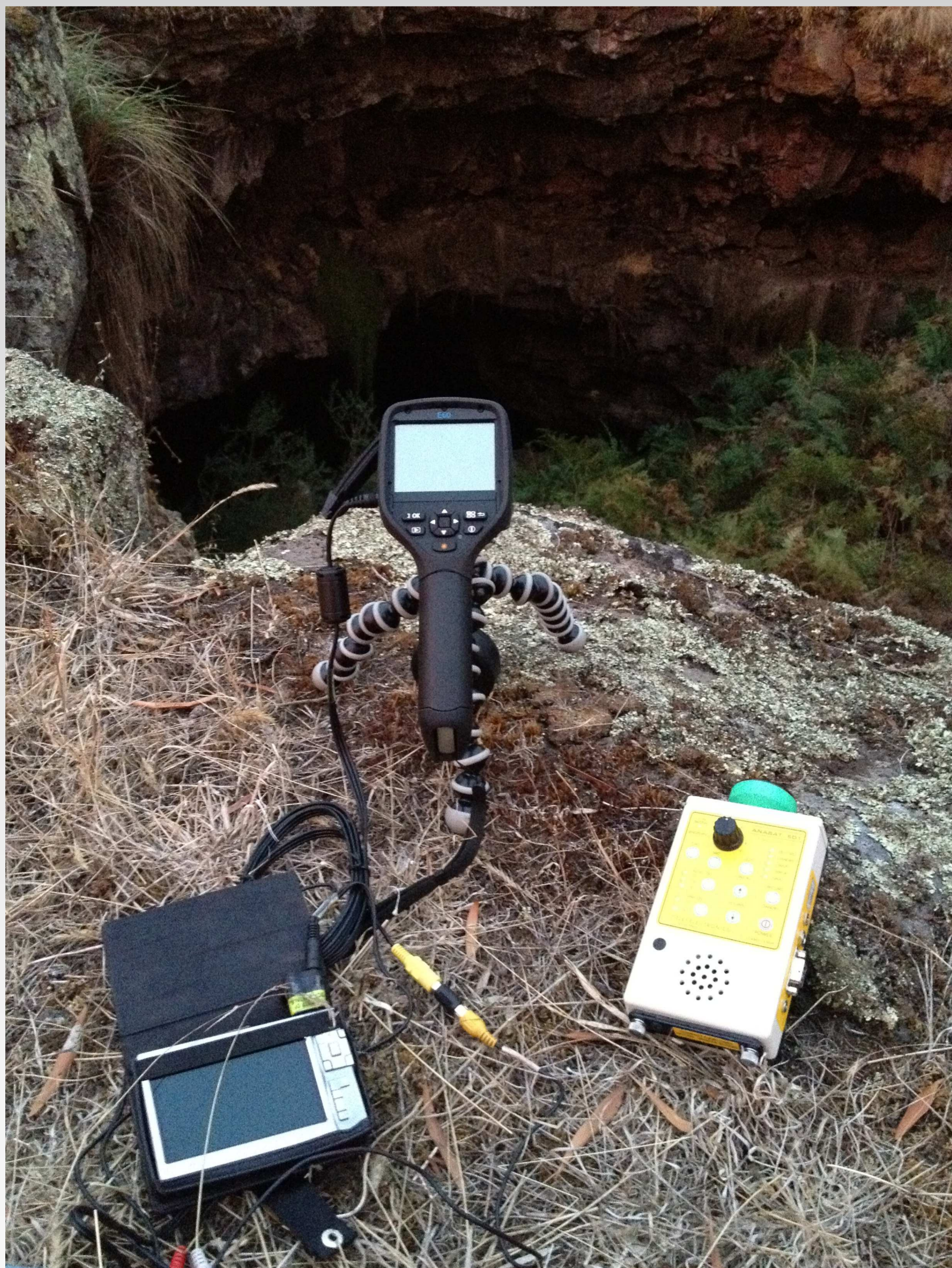
Figure 2. Highly portable thermal camera and DVR in situ at edge of collapsed lava tube at Bridge Cave (H-13). (Anabat detector on right).
